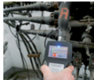
Online PD measurement on MV cable with the HFCT sensor.
