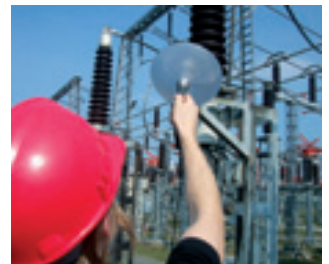
Outdoor insulation testing with the optional acoustic parabolic receiver.
