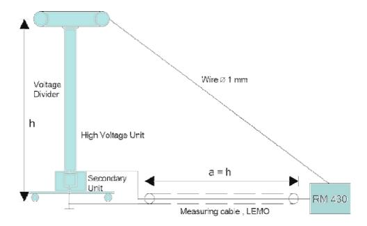
To measure a voltage divider the ratio meter RM430 is connected as shown above
